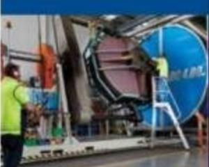
Sealite's marine buoys are manufactured using state-of-the-art rotational moulding equipment.
