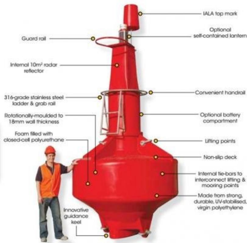
The NAUTILUS-2200 is a robust, rotationally-moulded polyethylene ocean buoy designed for offshore, port and coastal applications.
