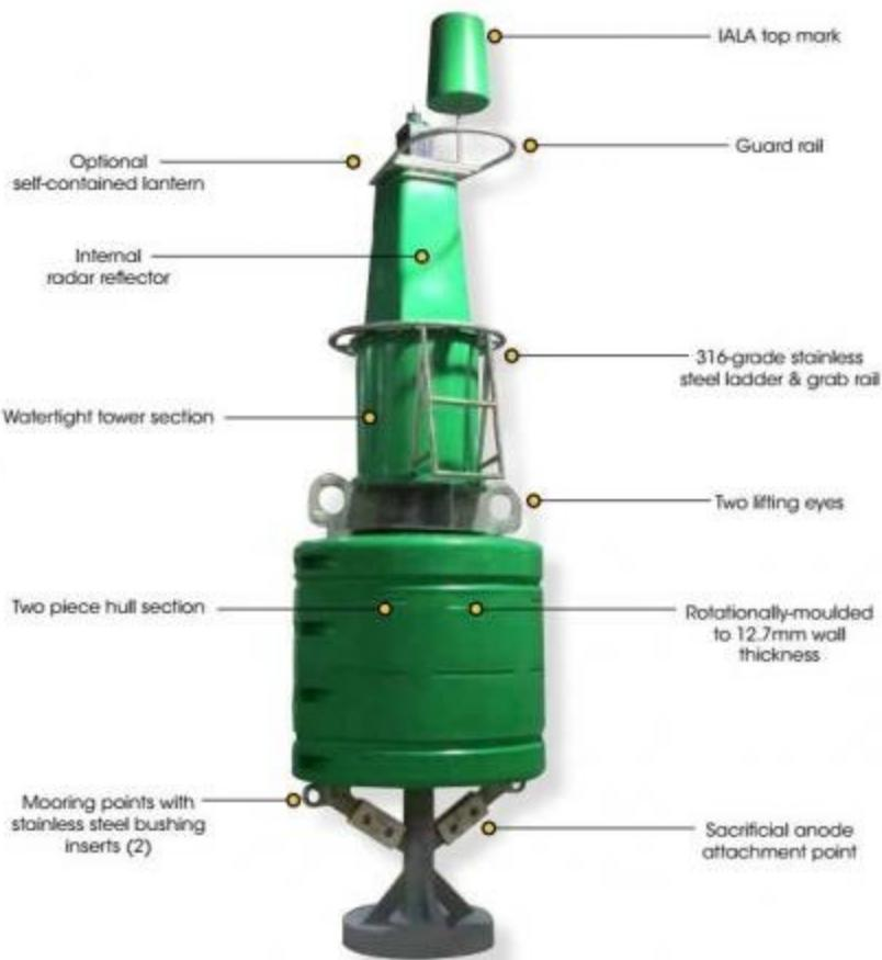
The TRIDENT-1400 is a rotationally-moulded navigation buoy with a float diameter of 1.4 meters and lantern focal height of at least 2.7 meters.
