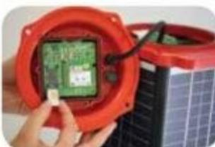
GSM module, SIM card & electronic hardware
